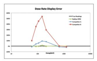
The energy compensated dose rate response of the RadEye SPRD ensures more accurate dose rate measurements providing greater assurance of personal safety.
